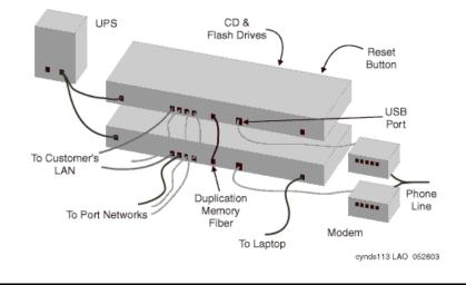
**UPS or power backup -** The S8700-series Servers always require power backup to avoid power problems, and to ensure graceful shutdown of the system processes if the power fails. The AS1 700-VA UPS provides approximately 30 minutes of power backup. Combinations of battery extension modules and a 1500-VA UPS provide up to 8 hours of power backup.
